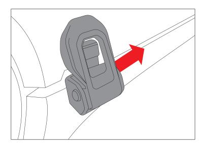
2. Remove Pivot Base from Aluminum Hood Catch assembly by unscrewing Binding Post.
