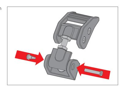
6. Adjust Aluminum Hood Catch by first releasing latch. With jam nuts loose, rotate latch clockwise to increase tension, or counter-clockwise to decrease tension. When properly adjusted, hood should contact and slightly compress Hood Bumper.
