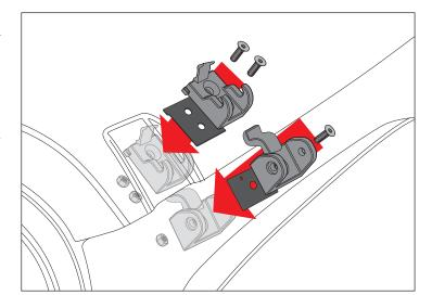
5. Re-install Aluminum Hood Catch assembly on Pivot Base using Binding Post removed in Step 2.
