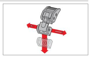
3. Fasten the catch to the hood. Fasten the pivot base to the fender.
