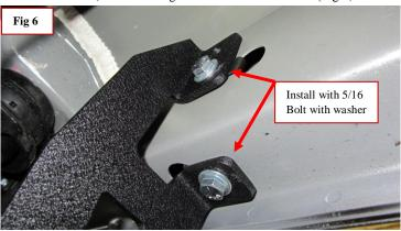
Step 5: Now with everything installed. Take a look at the board on your vehicle. There is a lot of adjustment in the kit to get the board where you like them. Adjust boards in and out and side to side with the slots on the bracket where board mounts. Adjust the front and rear brackets first and finish with the middle. Once the boards are in place to your liking, tighten all fasteners on the boards and brackets. This will complete your installation. Enjoy!
