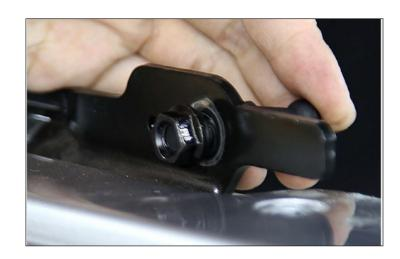
3. Remove the OE bolt from the frame but do not remove the OE bolt from the strap as this will ensure correct orientation when reinstalling the OE bolt.
