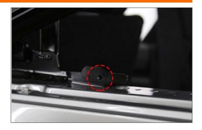
2. Install the supplied long ball stud and washers. Ensure the ball is pointing to the inside of the vehicle. Tighten hardware. Repeat on the other side.
