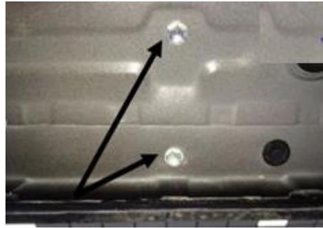
**Step 3:** Starting with the driver side, position step up to the body of the vehicle and align the brackets up with the factory mounting locations.
