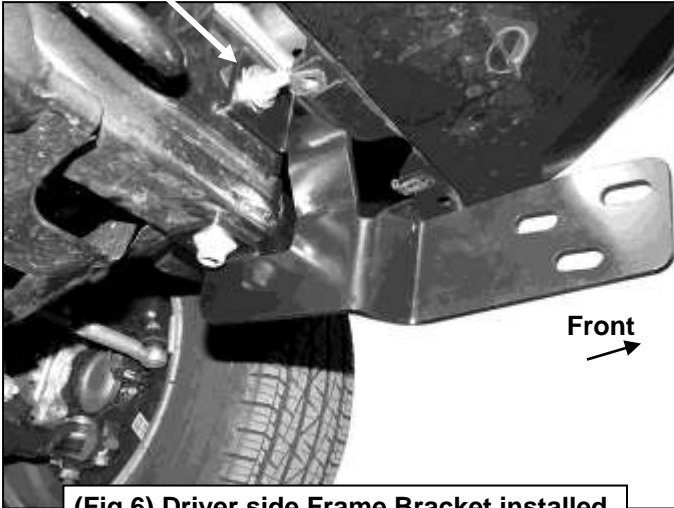
(Fig 6) Driver side Frame Bracket installed
