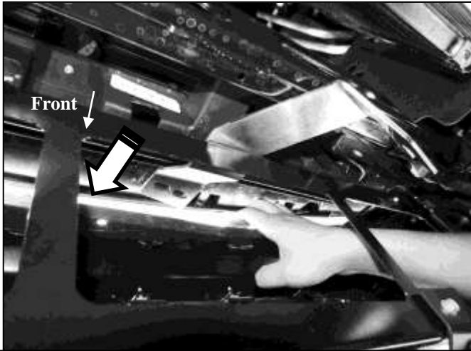
(Fig 10) Push down on the plastic trim on the bumper and carefully slide the front of the Bracket through the opening between the bumper and grille
