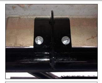
**NOTE:** The carriage bolt will start from the outside of the vehicle with the nut and washer on the backside.
