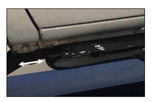
**Step 4:** Next, make a mark through each bracket mounting location onto the center of the pinch weld. Transfer you marks to the out-side of the pinch weld to center your holes that will be drilled.
