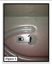
**Step 4:** Starting with the passenger side step, carefully lift up into position aligning the brackets to the mounting locations in the body of the vehicle and install hardware. Do not tighten all the way. **NOTE:** Some vehicles may require the use of additional nuts and washers for the lower portion of the mounting bracket which are supplied in the hardware kit.
