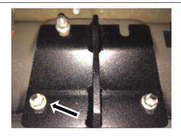
**Step 7.** After finial adjustment, tighten all three brackets at the main tube.
