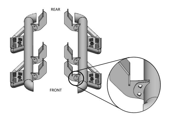
**Step 3.** If equipped, remove all 8mm nuts from the threaded studs and remove factory running board.
