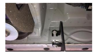
**Step 7:** After finial adjustment, tighten all three brackets at the main tube.
