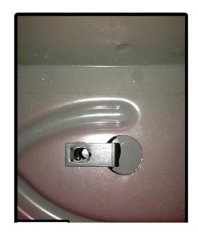
Step 5: Install the Nerf Step to the mounting locations in the body of the vehicle and install hardware. Do not tighten all the way. NOTE: Some vehicles may require the use of additional nuts and washers for the lower portion of the mounting bracket which are supplied in the hardware kit
