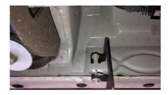
**Step 7:** After finial adjustment, tighten all three brackets at the main tube.
