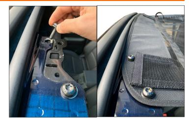
2. Insert metal hooks into the 2 factory metal tabs.
