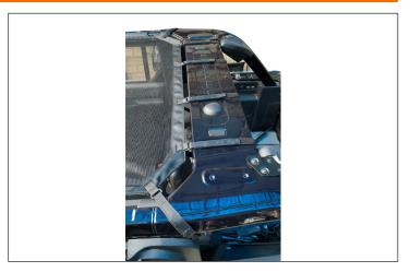
8. The flaps at the front corners can be secured open to maintain access to the windshield clamps.
