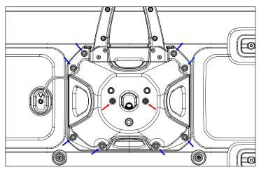
3. Place the tire carrier onto nearby table or cart. Remove the 4 screws holding the OE 3rd brake light to the tire carrier.
