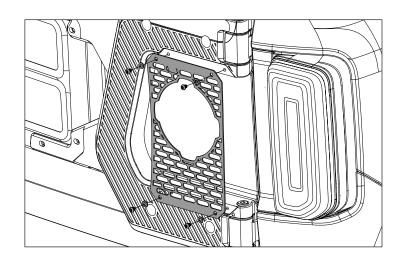
19. Using M8 x 15mm button head bolt(#10) and M8 washer(#7), attach antenna bracket to hinge casting.
