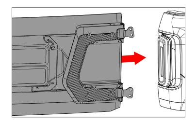
16. While gently holding up the tailgate, slowly close the tailgate. To compensate for added weight of the spare tire, we suggest adjusting the tailgate upward until the latch housing is making contact with the striker. Also, check the gaps between the tailgate and body panels.
