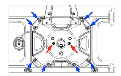
3. Place Tire carrier onto nearby table. Remove the 4 screws holding the OE 3rd brake light to tire carrier.
