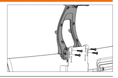
8. Reconnect OE camera to wire harness. Position OE camera housing into adjustable wheel mount bracket. Using supplied M6 flange head bolt, attach stud plate to adjustable wheel mount bracket.
