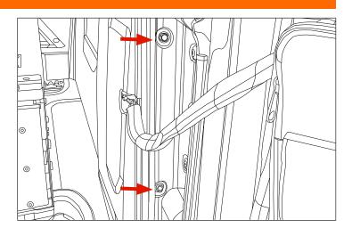
7. The tailgate strut is located on the bottom of the tailgate. Using a small flat head screw driver, lift retainer clip on tailgate strut. Gently pull strut away from ball bracket on tailgate.
