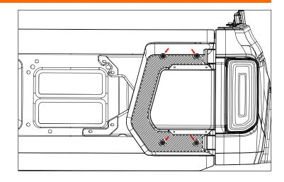
18. Using M6 button head bolt(#8) and washer(#9), attach logo mesh to hinge casting.
