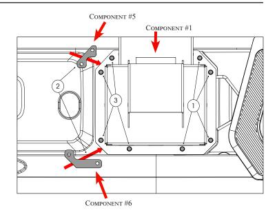
6. If you are installing the wheel mount <u>without</u> the Havoc hinge casting, loosely attach wheel mount to tailgate using supplied M8 hex head bolt(#7) and washers(#8).
