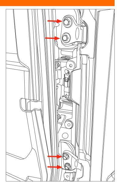
13. Using a T-45 Torx driver, remove the 4 bolts securing the upper and lower hinges from the tailgate.
