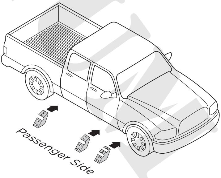
**4.** Align brackets with existing factory threaded holes in the rocker panel (4a). These holes may have black plugs in them that will need to be removed before installation. Fasten each bracket to the rocker panel using two (2) M8 x 30mm Hex Head Bolts, two (2) M8 Lock Washers and two (2) M8 Flat Washers (4b) per bracket.
