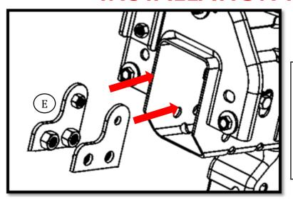
Insert frame horn nut plates (4)inside the vehicles frame horn. Be sure it is free of any debris. Repeat process for both sides.
