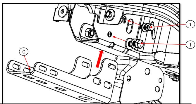
Install lower main bracket on to vehicle frame horn. The outer side of the frame horn will use (3) qty Hex Sems bolt M8 x 30mm. The inner side of the frame rail will use use (3) qty Hex Sems bolt M8 x 30mm. Repeat process for both sides.
