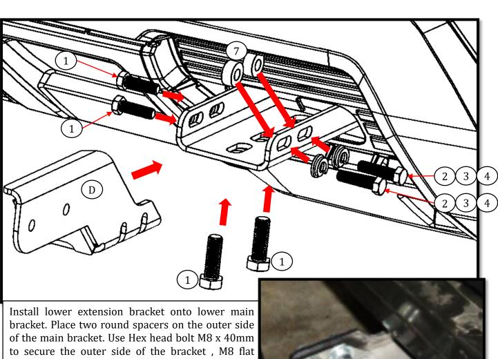
Install lower extension bracket onto lower main bracket. Place two round spacers on the outer side of the main bracket. Use Hex head bolt M8 x 40mm to secure the outer side of the bracket , M8 flat washer, M8 lock washer (2 per side), Hex Sems bolt M8 x 30mm to secure the inner side of the frame bracket. The bottom side can be secured using Hex Sems bolt M8 x 30mm (2 per side). Repeat process for both sides.
