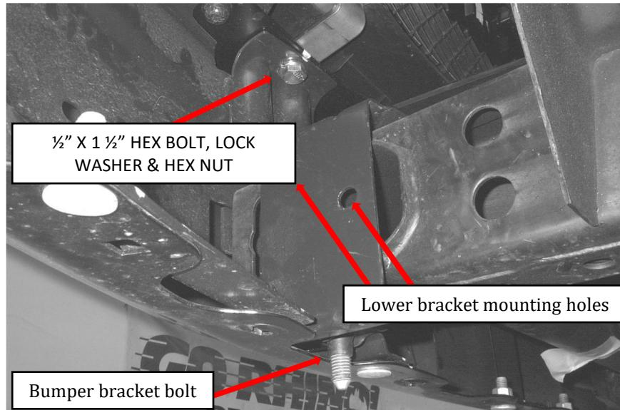
**STEP-5** LOCATE THE HOLES IN THE BUMPER BRACKET. THESE HOLES WILL SERVE AS THE LOWER BRACKET MOUNTING POINTS.
