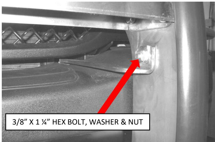
**STEP-8** ATTACH THE GRILLE GUARD ASSEMBLY TO THE UPPER BRACKETS USING THE 3/8 X 1" HEX BOLTS, LOCK WASHERS, FLAT WASHERS AND HEX NUTS.
