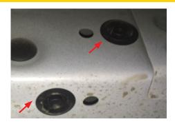
Step 2. Insert one (#4) 8mm barrel clip into each mounting hole by sliding the clip from the large hole and lining up the threaded part with the smaller hole. Make sure the flat side of the clip faces toward the outside of the body.
