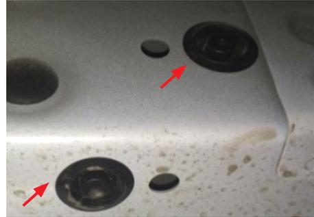
Step 2. Insert one (#4) 8mm barrel clip into each mounting hole by sliding the clip from the large hole and lining up the threaded part with the smaller hole. Make sure the flat side of the clip faces toward the outside of the body.
