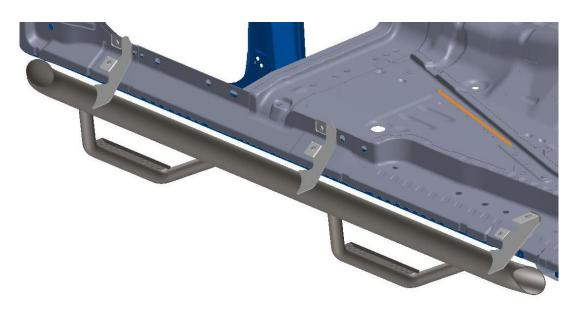
Step 5: Next, tighten the three lower bolts first following with the three upper bolts.Step 6: Repeat steps 2-5 with passenger side.Step7: Your install is now complete.
