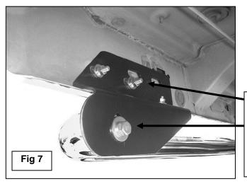
Narrow Double Bolt Plate uses (2) lower slots on Mounting Bracket (driver side 3-Door model only)
