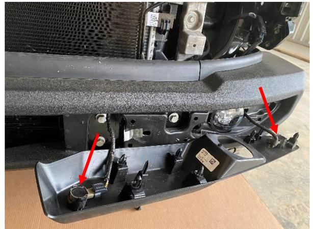
2. Once the plastic covers are removed, (a) locate the front sensor harness plug behind the driver side headlight and fender liner, (b) and unplug the harness. Now remove the 6 frame bolts using a 15mm socket, and the front bumper will come off.
