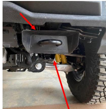
4. On the base model Bronco, the tow hooks may need to be cut out to complete installation.
