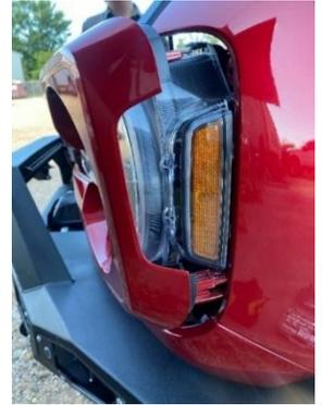
3. Now that the grill is free, disconnect your camera and camera washer spray line, above your passenger headlight. Once those items are disconnected, remove grill and set aside.
