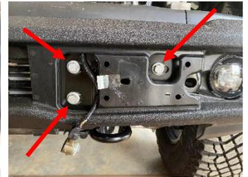
3. Once the bumper is off, detach the parking sensor wiring harness from the bumper, and locate the (6) bolts holding the skid plate, then remove the skid plate using the 15mm socket. With the skid plates off, remove both tow hook shrouds by sliding forward.
