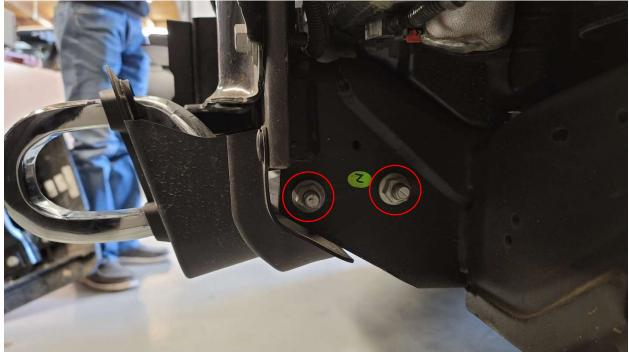
5. Finally remove the bolts holding the factory shackles circled in red. Save these bolts for the installation of your Bodyguard bumper.
