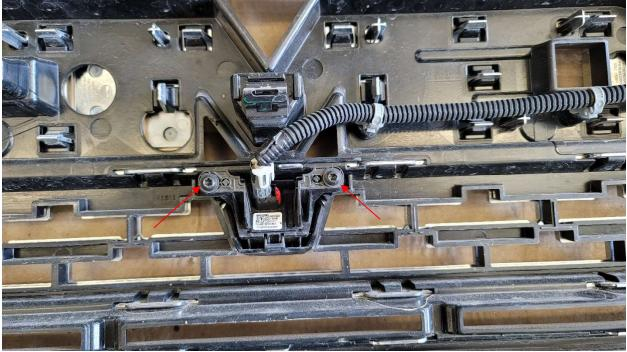
4. Remove camera from grille by removing the two torx screws shown above
