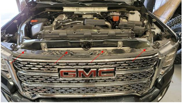
3. Next un screw the screws holding the grille to the truck.
