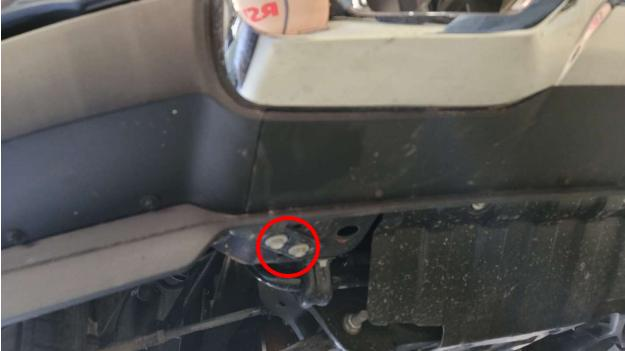
2. Remove the two bolts circled above. This will fully unbolt the bumper from the truck.
