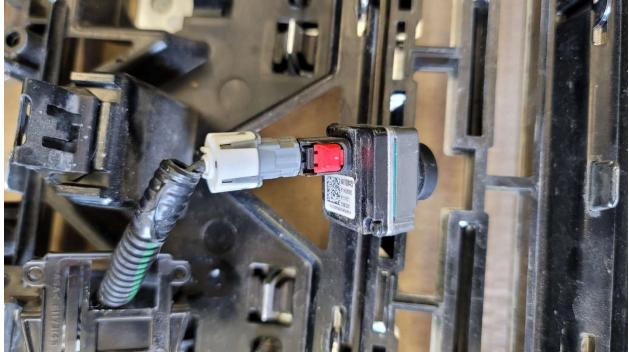
6. Disconnect camera from wiring harness. Place the camera in a safe place to be installed in the bumper in a later step.
