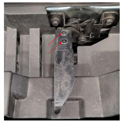
2. Remove torx screws from hood latch, and remove hood latch. Then remove the plastic cover above the grille.
