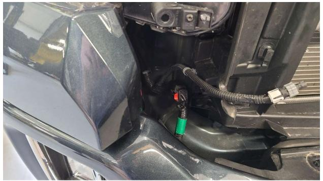
3. Once the bumper is loose this will help locate the fog light and sensor wiring harness plug. This is located on the passenger side. You may have to tilt or partially remove the factory bumper to better access this plug.
