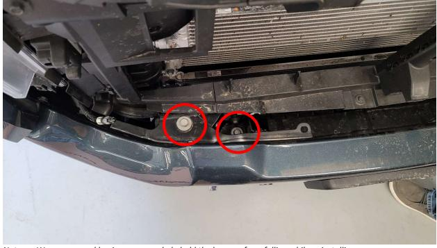
*Note: We recommend having someone help hold the bumper from falling while uninstalling* Remove the two bolts circled above. This will loosen the bumper from the factory truck mounts.
