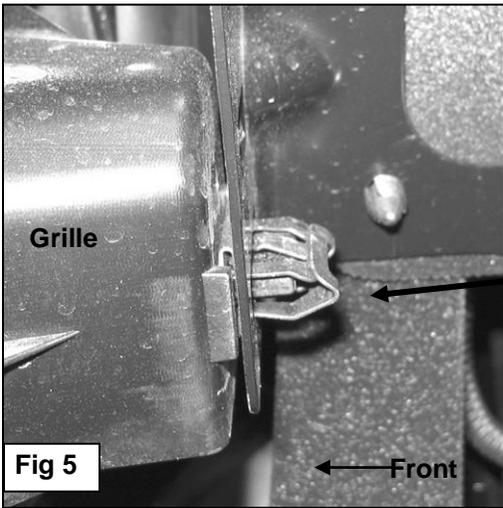
Close up view of retaining clip on back of grille insert
