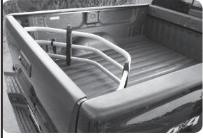
Before driving, secure BEDXTENDER by locking the provided strap buckles into the truck's tailgate latches. To release, pull tailgate handle. NOTE: Ensure that both buckles are properly locked into the latches by pulling up on each strap.
