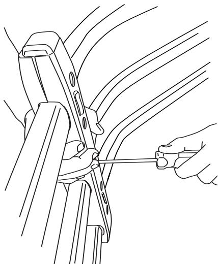
**8** NOTE: The inside of the upright is stepped to fit correctly around the small and large diameter tubes.
