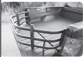
With the tailgate open, place BEDXTENDER pivot pins into the left and right mounting brackets. Rotate to 45 until it drops into place, then lower onto the open tailgate.
