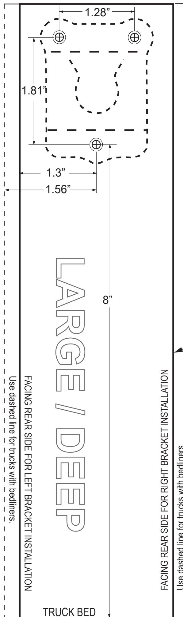
Drill template for BEDXTENDER HD™ mounting brackets
