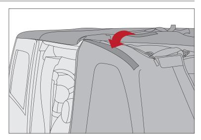
25. Insert remaining side window plastic retainers into groove of body tub. Repeat for opposide side.
