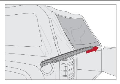
27. Install metal hook on end of rear straps into body tub through cutout in rear panel and tighten. Repeat for opposite side.
