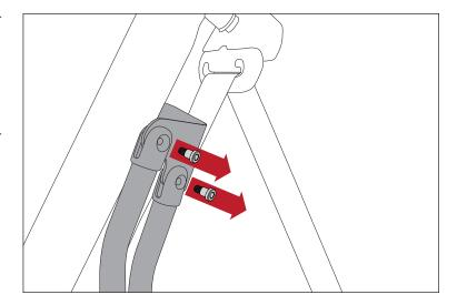
2. Remove metal soft top mounting brackets attached to roll bar in cargo area.
