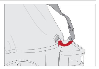
28. If desired, rear window can be rolled upwards, secured with two rear straps, and fastened to top with snaps located under top flap.
