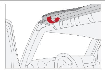
9. Hook side plastic retainer over rear door surround and hook into groove over rear door. Repeat for opposite side.
