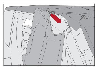
21. Pull bottom plastic retainer of side window into side groove of body tub. Repeat step 19 - 21 for opposite side.
