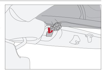
7. Ensure header is flush with windshield and screw plastic knob into header on each side of vehicle.
