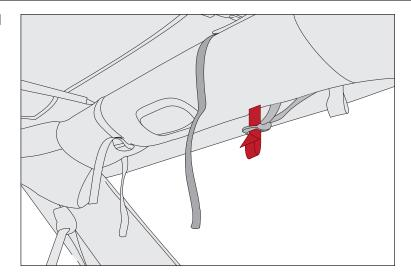
13. Loop rear side strap around rear sport bar, moving toward outside of vehicle.
