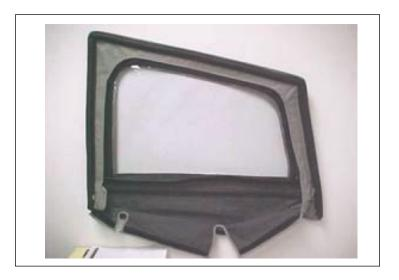
11. Unzip the Door Skin Window. Insert the frame into the upper rear corner of the door skin and then insert the Frame into the upper front corner of the Door Skin. Press down the Velcro to secure the frame bar.
