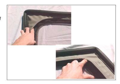
12. Insert the lower front corner of the Frame into the Door Skin (tight fit). Wrap the Velcro around the Frame that runs the length of the bottom and secure. Make sure the three legs of the Frame are seated in the 3 cut-away parts of the Door Skin. Close the 2 large and 1 small flaps on the bottom of the Door Skin. Door Skin is now assembled.
