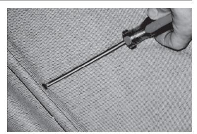
5. Lower soft top and remove screws that fasten soft top fabric to bottom corners of header. Set screws aside for later use.
