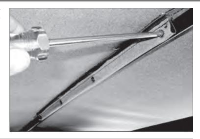
4. Unfasten hook and loop retainer that secures top to bow above roll bar and lower soft top.
