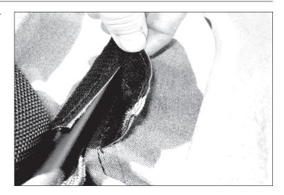
11. Insert rear corners of soft top into belt rail.
