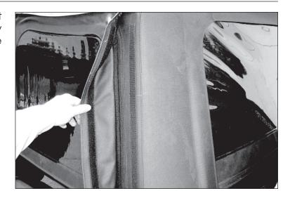
2. Release windshield latches on front header. DO NOT lower top at this point. Pull down and out on corners to release top from belt rail. Repeat for opposite side.
