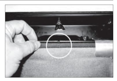
8. Drape new fabric over back of vehicle and lower frame assembly. Wrap fabric around corners of header assembly. Ensure fabric is tucked between lip of header as shown. Reattach plastic tab to header using screws removed in step 5.
