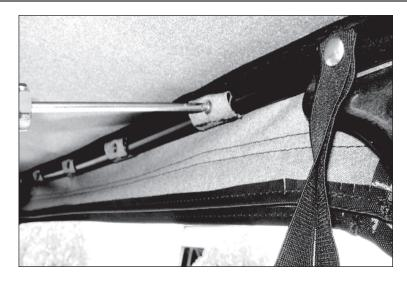
10. Reattach hook and loop retainer around front bow above center roll bar.
