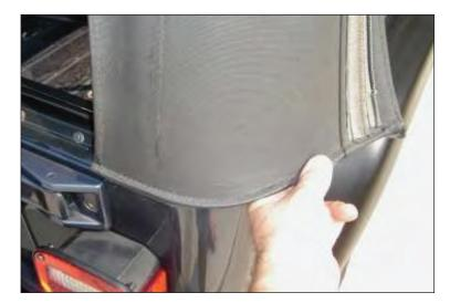
11. Wrap and fasten hook and loop strips around center bow.
