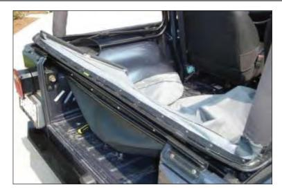
7. Lay new soft top fabric in rear of vehicle with bottom side up. Ensure plastic strip on fabric is facing up and aligned with front edge of windshield header. Locate round hole that marks center of plastic strip and install first screw to ensure fabric is centered on header. Install remaining screws removed in step 6.
