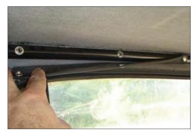
5. Lower soft top onto tailgate. Remove screws that fasten soft top fabric to corners of windshield header and set aside for later use.
