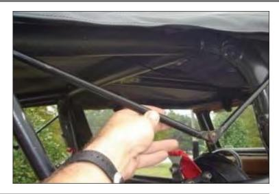
4. Pull down and out on corners to release top from belt rail. Repeat for opposite side.
