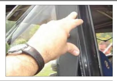
13. Slide plastic strip on bottom of side window into belt rail. Start at one end of window and work along vehicle to other end. Close top and rear zippers on side windows.
