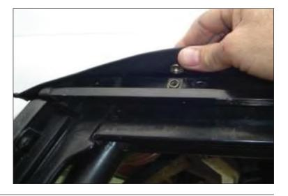
17. Remove fabric upper doors from vehicle. Using razor blade, cut stitching on old door covers and remove from frame.
