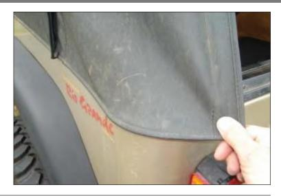
10. Pull bottom rear support bow back until it snaps into notch in side rail.
