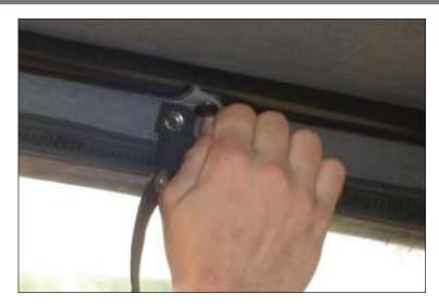
7. Insert front top plastic strip into windshield channel retainer.
