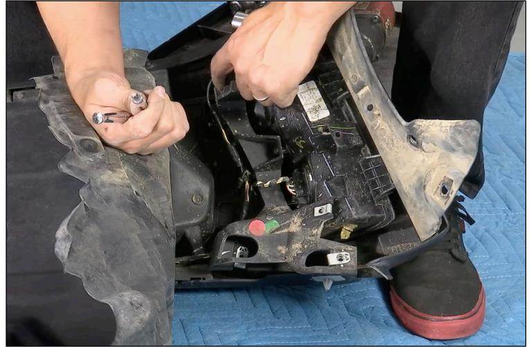
5. Using a T25 torx bit remove the four screws holding the rear brace to the light. Next use a T30 torx bit to remove the remaining screws. With all the screws removed the rear brace can be removed.
