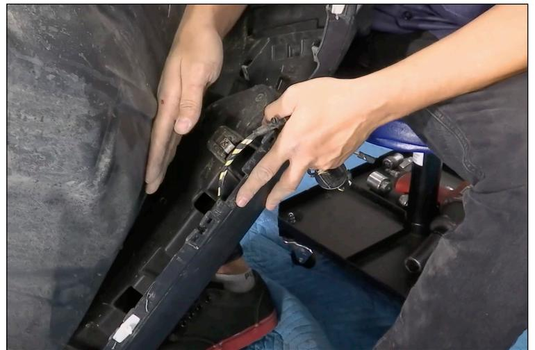
9. Now remove the plastic surround of the light. There is a clip holding the plastic to the fender. Pry and remove this clip. Next use a utility knife or snips to cut the plastic surround to release the side closest to the inside of the fender.
