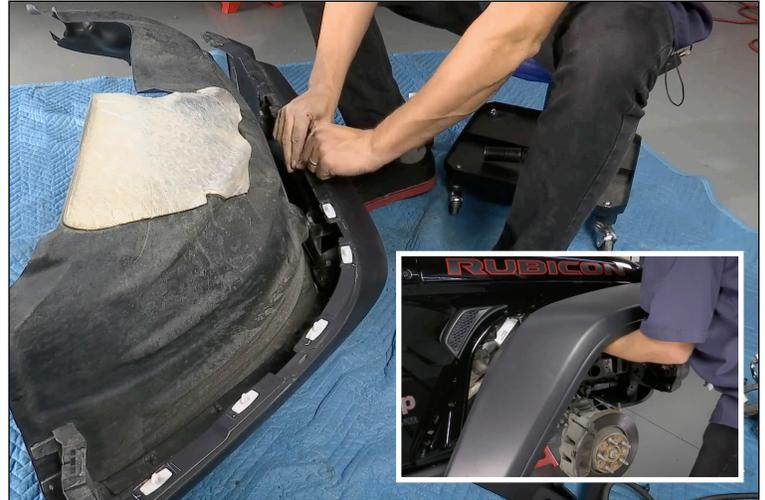
14. Place the Chop Bracket into place. You are using it to mark the areas you must trim further. Remember the phrase "Less is Best" concerning cutting. Trim and return the bracket in place to check your cut, trim more as needed. This will assure the tightest and cleanest fit. Remove any sharp edges with sandpaper if needed.
