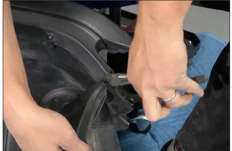
11. The new Chop Bracket has a section where adhesive tape will be applied. We must remove a section of the inner structure to meet the fender to the bracket adhesive. Be very cautious with the tools and the depth of your cut. You DO NOT want to cut through your fender. Use a utility knife or cut off wheel to make the cut. See the red dotted line in the picture of the cut.
