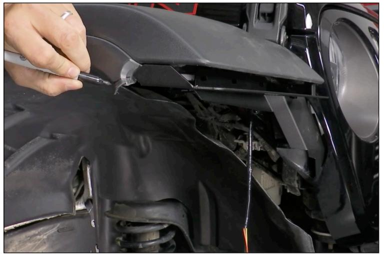
15. Now install the bracket with the 3M tape to the Chop Bracket using the carriage bolts, washers and nylock nuts provided. Do not fully tighten, allow the bracket to slide up and down. This will allow you to adjust the height to assure the adhesion meets the fender.
