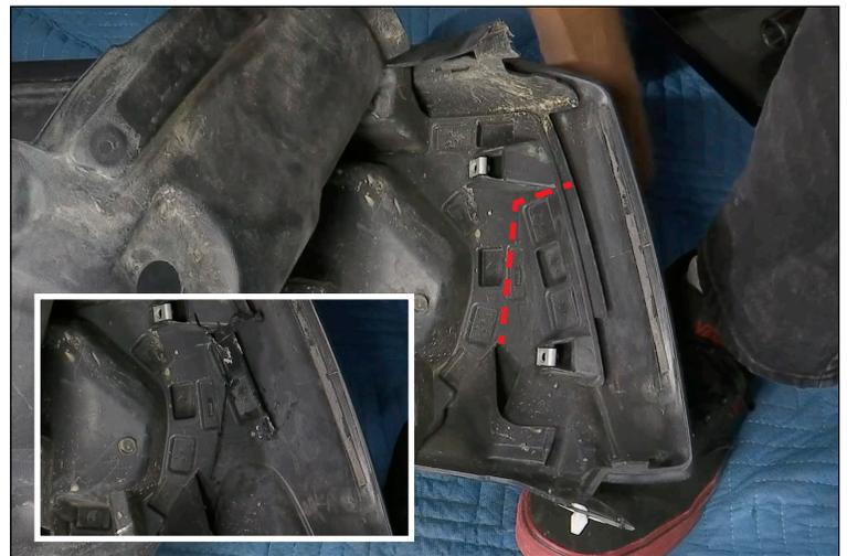
12. Each light is marked L (Passenger Side) and R (Drivers Side). Take the light and plug to the OE harness. Be sure to press the gray tab in after the harness is fully pushed in, this will lock it together. Lay the wire of the light in the fender braces. Take tie wraps and secure the wire to the braces.
