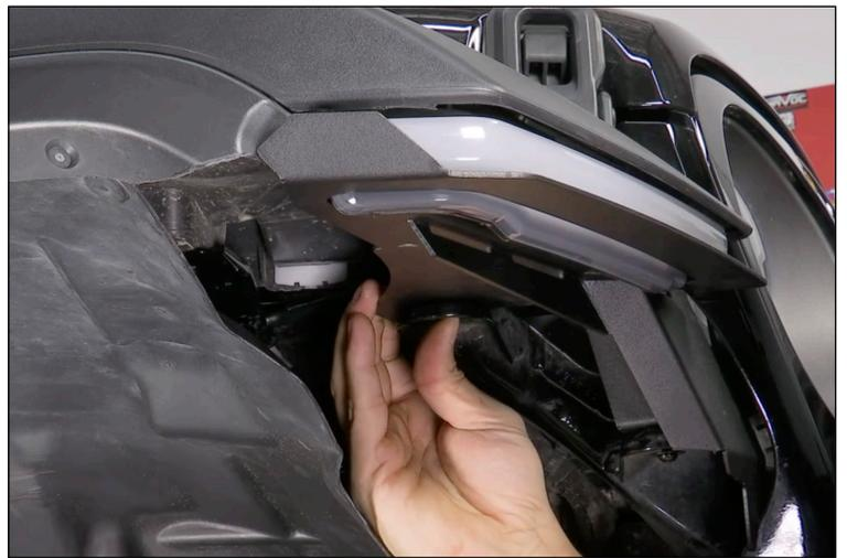
18. Attach the inner fender to the body of the Jeep using the same hardware (bolts and push rivets) you removed earlier.
