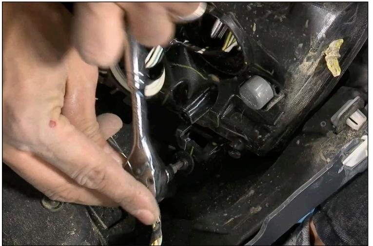
6. With the rear brace removed it exposes another T30 torx screw that holds the side marker light in place. Remove this screw and remove the marker light.
