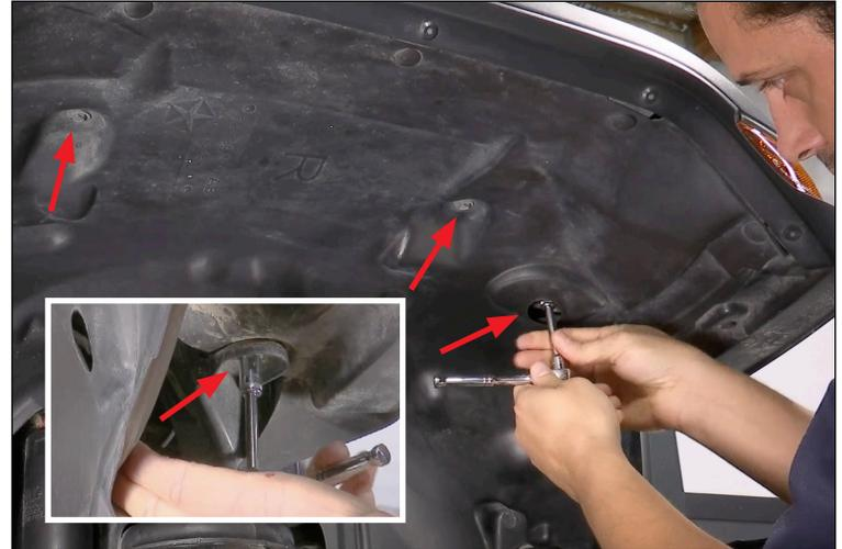
2. Use a pry tool to remove the push rivets holding the liner to the body of the Jeep.
