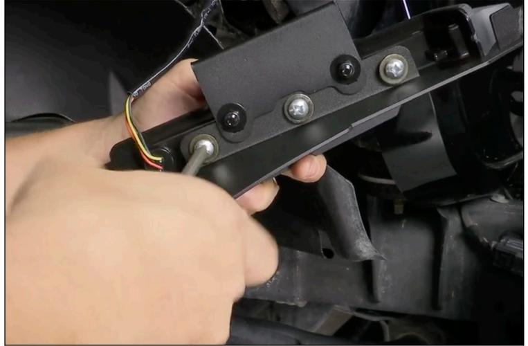
17. Apply adhesive promotor to underside of the fender. Peel the backing from the 3M tape. Place the bracket into place. Use the 2 button head bolts, washers and nuts to attach the bracket to the two fender mounts. With mount fully tight reach back and push the adhesive bracket up and press the top of the fender to secure. Then tighten the nuts of the bracket with the adhesion.
