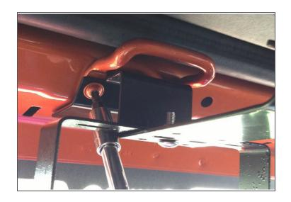
5. Replace center plastic windshield frame cover. Install CB Mount, radar detector, or GPS device using M5x15 bolts and Locking Hex Nuts.
