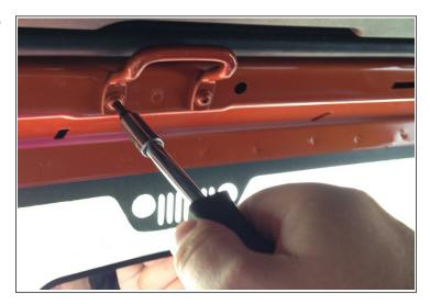
3. For **2007-2010** model JK's: insert the Well Nuts into the newly drilled holes in the sheet metal. If drilled holes are too large to snuggly fit Well Nuts, secure with small amount of super glue.
