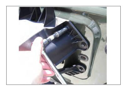
8. Install the CB Antenna Mount using the supplied hex bolts, lock washers, and flat washers. Torque the bolts to 10 ft-lbs. Remount the spare tire after CB Antenna installation is complete.
