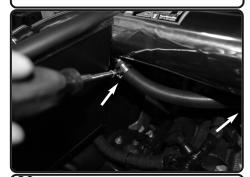
**20.** Secure the crankcase line to the fitting on the intake tube. Tighten both clamps using 8mm nut driver.
