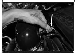
**23.** Re-connect the temperature sensor harness.
