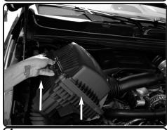
**4.** Lift up and remove the air box assembly out of the vehicle.
