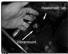
**12.** Secure the bracket using provided M6 vibramount and M6 nut under plastic. This will be used for the intake tube.
