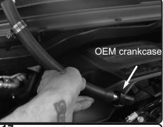
**17.** Now install the crankcase line to OEM plastic crank case line from step 7. Make sure you hear a click.
