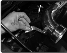
**19.** Position for best fit, Secure and tighten backet using provided M6 nut and fender washer.
