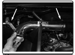
**18.** Install the intake tube and position the bracket to the vibramount and to the elbow hose. Do not tighten.
