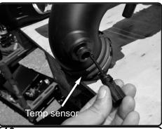
**13.** With flat head screwdriver, carefully turn and remove the temperature sensor out of the OEM intake tube.
