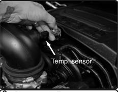
**2.** Disconnect the Temperature sensor harness.
