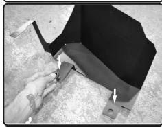
7. Install the provided 2 6014 grommets to the holes on the heatshield.
