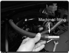
**16.** Attach the 17mm hose to the machined fitting with clamps provided.
