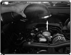
**5.** Pull back the intake tube from the throttle body.
