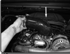
**15.** Install the elbow hose assembly to the throttle body. Do not tighten.
