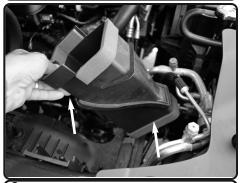
**6.** Carefully lift up and remove the front plastic scoop
