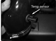
**14.** Install the temperature sensor grommet into the hole on the elbow hose. attach the clamps to the elbow hose.
