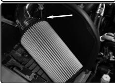
**21.** Install the filter to the intake tube.
