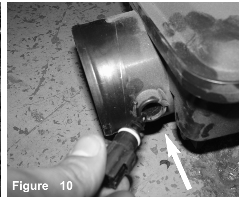
Figure 10 Turn the temp sensor, and pull back from the resonator and remove.
