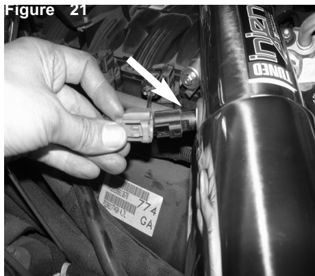
Connect the temp sensor harness.
