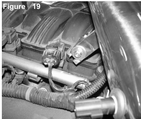
Figure 19 Secure the bracket using provided M6 nut and fender washer.
