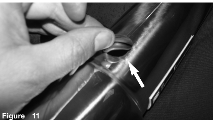
Figure 11 Install the provided grommet into the hole that is on the intake tube.
