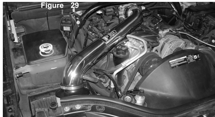
Connect the crank case line to the fitting on the intake tube.
