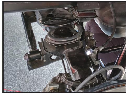
2. Install the billet track bar using the factory hardware and torque to factory spec using a 19mm. [FIGURE 3 & 4]
