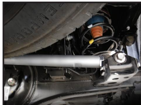
**3.** To adjust, loosen jam nuts using a 1-5/16" and turn the billet track bar. Once the differential is centered under the frame, torque the jam nuts to 180 ft-lbs.
