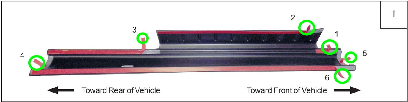
Peel back 2" of tape liner from each flange. Using a marker, number the tape tabs as shown:
