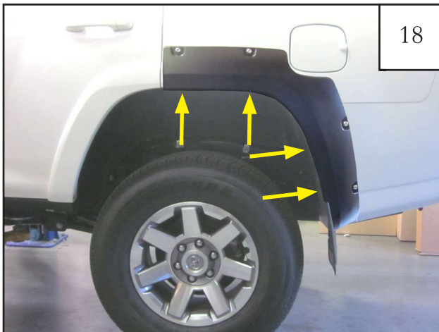
Ensure flare is positioned properly, then apply inward pressure on the flare at each hole location while tightening each screw.
