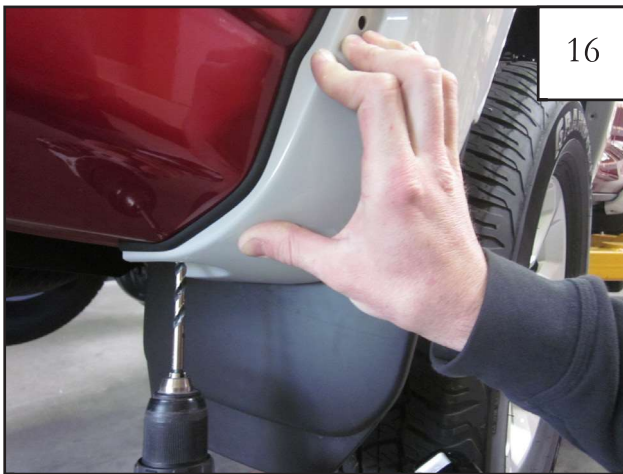
Drill a 5/16" hole in the lower rear hole location. NOTE: Press inward on the flare when drilling to ensure proper hole location.
