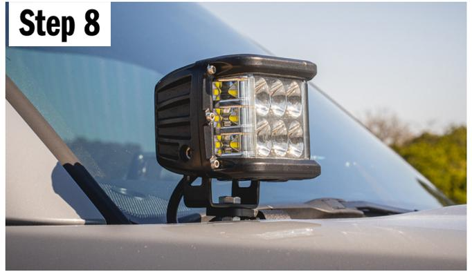
Tighten all the bolts and close your hood. Check for clearance and make any necessary adjustments if needed. Lastly you want to aim your lights to the desired spot, then tighten the pod the u-bracket, and u-bracket to the ditch mount.
