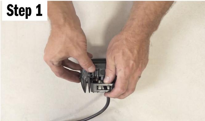
Install pod u-bracket to the LED pod. Use included hardware and tools that came with your pod.
