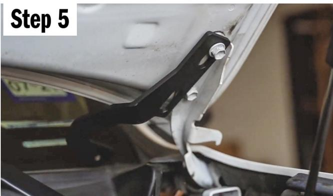
Remove the nut/bolt and move the mount in place, then put the nut/bolt back in place, snug but not tight.
