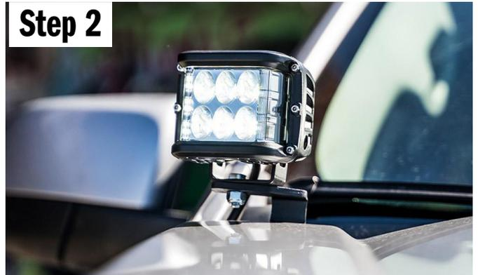
Install your pod to your ditch mount in the correct direction. If you have side shooter style pods, make sure you have the correct pod on the correct bracket. For example, make sure the passenger side pod is on the passenger side bracket. For side shooters, make sure the side LEDs are pointing away from your hood.
