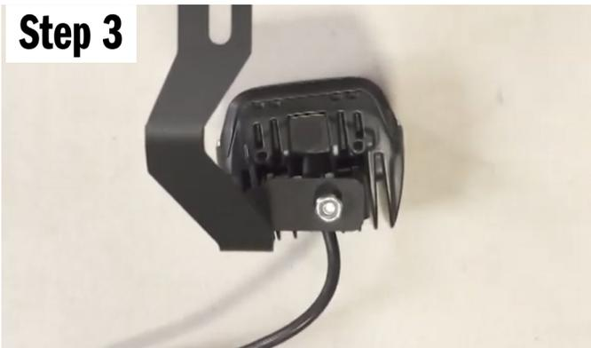
Use the hardware that is included with your ditch mounts to connect the pod to the mount. Do NOT use the hardware included with your pods. Put the bolt through the u-bracket, then through the ditch mount, then install your lock nut on the bottom. Tighten so it doesn't flop around, but leave loose enough to make light adjustments after mounting to your vehicle.
