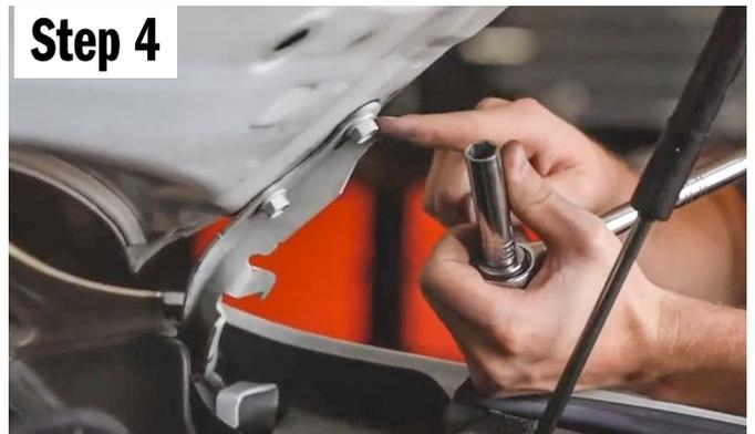
Now we are going to install the bracket to your vehicle. Start by loosening the top nut or bolt that holds your hood in place.
