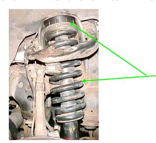
INSTALL THE STRUT ASSEMBLY INTO THE FACTORY MOUNTING LOCATION.
