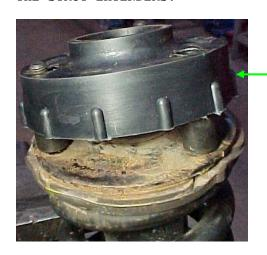
URETHANE SPACER BEING INSTALLED OVER THE STRUT EXTENDERS.
