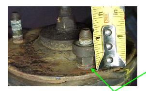
FACTORY NUT INSTALLED 3/4" ABOVE THE TOP OF THE STRUT MOUNT WITH HEX SIDE DOWN SO IT CAN BE USED AS A GUIDE TO TRIM THE STUD OFF.
