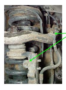
REMOVE THESE TWO BOLTS THAT HOLD THE BRAKE LINE AND ANTI LOCK BRAKE WIRE TO THE STEERING KNUCKLE AND UPPER CONTROL ARM, SAVE THIS HARDWARE.
