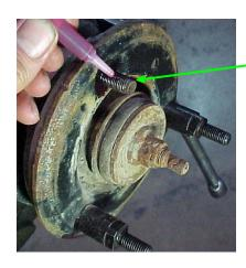
HIGH STRENGTH THREAD LOCKER BEING APPLIED TO LOCK THE NEW STRUT EXTENDERS IN PLACE. B. INSTALL THE THREE SUPPLIED STRUT EXTENDERS PER STRUT AND TIGHTEN USING A 5/8" WRENCH.
