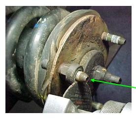
NOTE: THE STUD TRIMMING PROCEDURE MUST BE COMPLETED SO THAT THE NEW STRUT EXTENDERS WILL SEAT FLAT AGAINST THE TOP OF THE STRUT MOUNT WHEN INSTALLED AND TIGHTENED.
