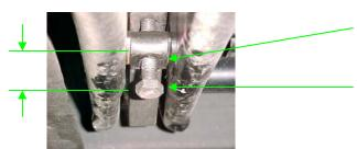
TORSION BAR ADJUSTER BOLT RETAINING PLATE.
