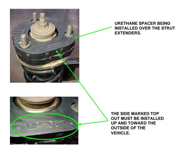
17. STRUT AND NEW STRUT SPACER ASSEMBLY INSTALLATION.
