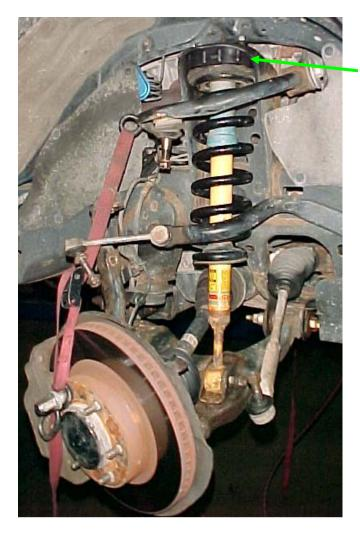
STRUT WITH NEW LEVELING SPACER ASSEMBLY MOUNTED TO THE TOP.
