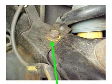
REMOVE THE BOLT HOLDING THE ANTI LOCK BRAKE BRACKET AND LINE FROM THE UPPER CONTROL ARM SAVE THIS HARDWARE.
