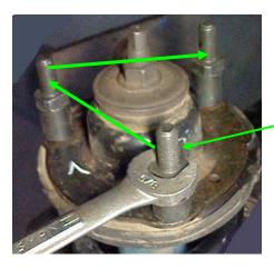
STRUT EXTENDERS BEING INSTALLED OVER THE FACTORY STRUT UPPER MOUNTING STUDS.
