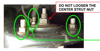
LOOSEN THE THREE OUTER UPPER STRUT MOUNTING NUTS.
