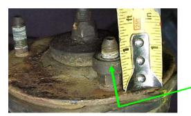
FACTORY NUT INSTALLED <sup>3</sup>/4" ABOVE THE TOP OF THE STRUT MOUNT WITH HEX SIDE DOWN SO IT CAN BE USED AS A GUIDE TO TRIM THE STUD OFF.
