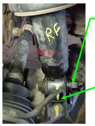
HARDWARE HOLDING LOWER STRUT MOUNT TO THE LOWER CONTROL ARM
