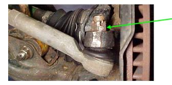
REMOVE THE TIE ROD COTTER PIN, TIE ROD NUT AND REMOVE TIE ROD FROM THE SPINDLE. 6. SUPPORT THE LOWER CONTROL ARM, REMOVE THE FACTORY UPPER BALL JOINT COTTER PIN, LOOSEN THE UPPER BALL JOINT NUT, TAP ON THE STEERING KNUCKLE WITH A MALLET TO POP THE UPPER BALL LOOSE. REMOVE THE UPPER BALL JOINT NUT AND REMOVE THE UPPER BALL JOINT FROM THE STEERING KNUCKLE, SAVE THE BALL JOINT NUT FOR REASSEMBLY.
