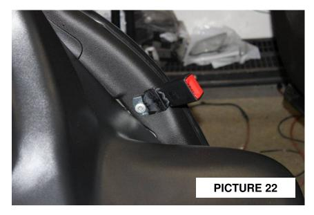
• 25) Attach the seat belt clips to the front screen. Place them as far out, towards the doors as the seat belt length will allow. As seen in picture 23. Peel the back of the adhesive and press to the screen. Attach seat belts.
