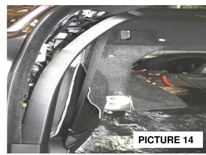
Retractor accessible, see pictures 15A and 15B; remove them from the vehicle using a 50Torx drive. Keep the hardware from the Shoulder Belt Loop, as you will be using this to install the Aedec Shoulder Buckle. Repeat for the other side.
