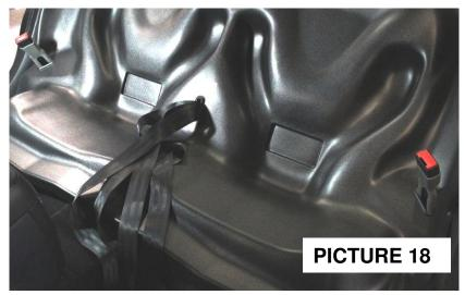
19) Fasten the Aedec Center Belts to the Seat belt bracket using the supplied 1/2"x 1-1/4" bolt, two 1/2" washers and one 1/2" Nylok nut. See picture 20.
