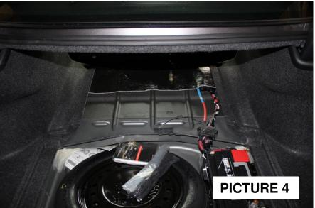
flaps pulled up; the seven 18mm factory nuts that need to be removed should all be exposed (2 on each outside; see picture 5, and 3 in the middle of the seat). Remove the nuts but keep the fasteners as they will be used later. The back seat is a 60/40 split seat. With the seat completely detached from the vehicle, separate it and remove it from the car.
