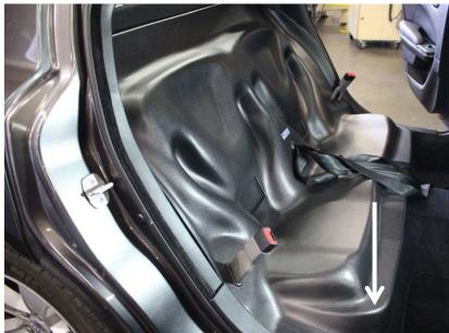
• 23) Using the supplied 1/4"x 1" HWH screws and 1/4"x1" flat washers, secure the seat to the vehicle in the recessed/dimpled areas on the back of the seat. On the two dimples on the back of the seat screw straight towards the back of the vehicle. Using the supplied 1/4"x 1" HWH screws with the 1/2" bibb washers already attached; attach the seat to the vehicle at the two recessed area on the bottom of the seat insert the screws in a straight downward fashion. See picture 22.
