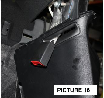
17) Mount the Aedec Seat Belt Bracket to the vehicle as seen in picture 17. Use the factory hardware to fasten the bracket down. Note the brackets are marked Left and Right.
