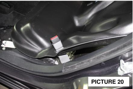
• 21)With all the buckles and belts securely fastened into the vehicle; position the seat so the front bottom lip fits snug up to the vehicle. And the back of the seat fits as high and as far back as possible. The edge of the seats should follow the contour of the trim on the vehicle. This will not be exact, but there should not be any gap left between the seat and the vehicle.
