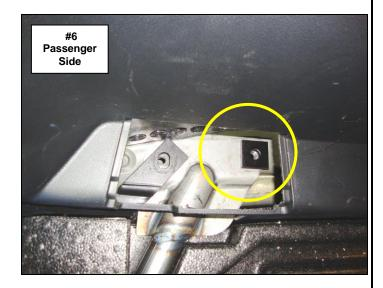
**Step-7** Position the base of the Electronics Tray right support bracket on top of the Aedec floor strut lower mounting flange and the supplied spacer, align the holes and reinstall the (2) factory bolts, (Photo 7). Snug, do not tighten the bolts.
