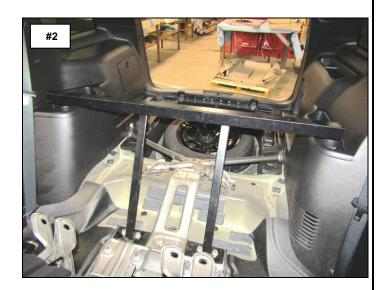
**Step-4** In the cargo area, remove the left and right plastic access cover, and remove the (4) bolts two per side securing the structural reinforcement X-Brace using a 15mm socket and ratchet, (Photo 3 & 4). **Note:** The access covers will not be re-installed.
