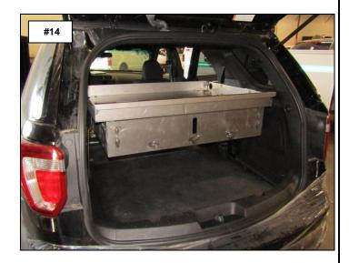
**Step-17** Reinstall the front and rear section of the cargo floor.
