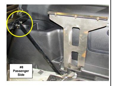
**Step-9** Repeat Steps 5-8 to install the left Aedec floor strut and Electronics Tray left support bracket, then tighten all factory bolts securing the left and right support brackets and Aedec floor struts.
