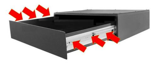
**Step-2** With assistance place the equipment security box on top of the false floor cover. Align the attachment holes in the base of the equipment security box with the holes in the false floor cover and rivet-nuts in the false floor brackets, Attach the equipment security box to the false floor cover and brackets using the (4)  $\frac{1}{4}$ " x  $\frac{3}{4}$ " button head screws and (4)  $\frac{1}{4}$ " flat washers supplied with the false floor. Tighten the screws.
