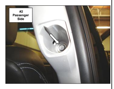
Step-3 Position the spacer tube inside the lower opening in entry assist handle and secure the passenger side B-pillar bracket using (1) M5 hex bolt and (1) M5 flat washer, (Photo 3 & 4). Leave the bolt loose for final adjustment.
