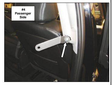
**Step-4** Remove the rear plastic trim cover from the front seat outer seat track rail and from the side area of the same track rail, unsnap the side area trim and slide forward to remove, **(Photo 5 & 6).**
