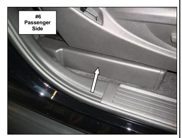
**Step-5** Remove the Torx head bolt securing the rear of the passenger side outer seat track. Align the attrachment hole in the passenger side foot bracket with the seat track and reinstall the factory bolt. Leave the bolt loose for final adjustment, **(Photo 7 & 8)**. Repeat the above steps to install the driver side B-pillar bracket and foot bracket.
