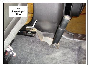
**Step-6** With assistance move the partition into the vehicle through the rear door. Lean the partition back, align the partition legs with the foot brackets then slide the partition legs over the foot bracket stub tube.
