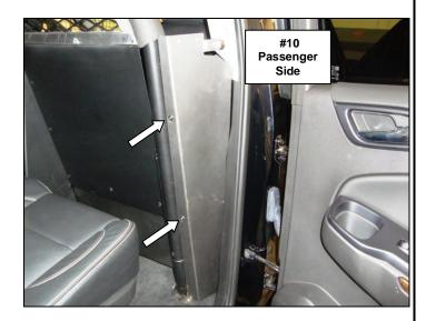
**Step-9** Attach the passenger side upper filler panel to the mounting tab and to the lower filler panel using (3) ¼" x ½" nylon slot head screws, **(Photo 11).**
